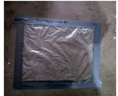
**ASTM Standard F1869**, is used to measure the moisture vapor emission rate of concrete subfloors using anhydrous calcium chloride. This method is appropriate only for horizontal concrete, particularly floors. In summary, a canister containing calcium chloride is weighed and placed on bare concrete, and then covered with a plastic dome and sealed. After three days, the canister is re-weighed to determine the moisture emission rate.
