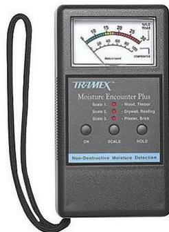
**All-in-One Moisture Meters** utilizes both previous types of moisture meters. This type of moisture meter gives the user the capability of identifying problem areas and pinpoint the exact location where moisture damage or buildup is occurring. %MC measurements can be taken on wood and non-wood substrates.
