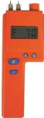
**Pin-less Moisture Meters**, or non-destructive/non-invasive moisture meters, operate on the surface without penetrating it. This type of moisture meter provides measurements for wood and other substrates, such as concrete and gypsum. Pin-less moisture meters are commonly used on concrete subfloors and flooring, and other areas to identify possible moisture buildup behind finished surfaces.
