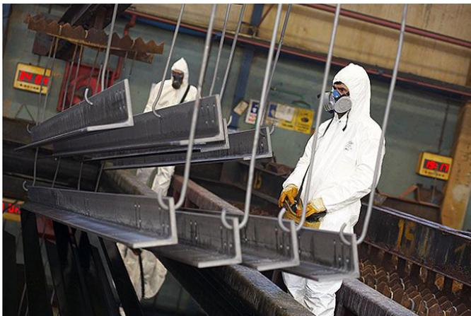
galvanizing or after-fabrication, heavy duty galvanizing. This process results in the highest level of protection and is commonly specified for highly corrosive interior and exterior environments.
