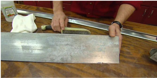
appropriate cleaner-degreaser followed by a Brush-Off Blast (SSPC-SP16) or chemical etching solution. If an etching solution is used, it must be thoroughly rinsed prior to applying any coating. Once these steps are completed, the galvanized steel can be coated.
